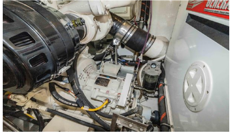
Air Intake, Transmission and Generator
