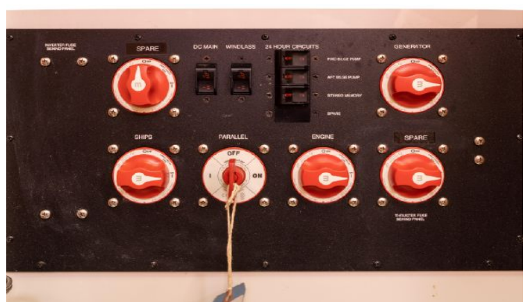
Battery Isolation Switches Conveniently Accessible
